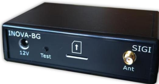
On the back are the connectors for 12V DC power supply, test button, SIM card push-in holder and GPRS mobile network antenna connector.
