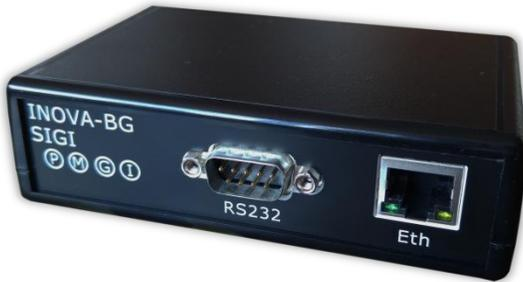
On the front panel there is RS232 and Ethernet connectors and four LED indicators:
